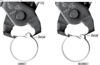
The nose of the plier should be firmly seated under the assembly bump and lock latch. If the pliers are not kept square as you close the clip, the clasp may have an offset. Use the pliers to correct the clasp alignment.
